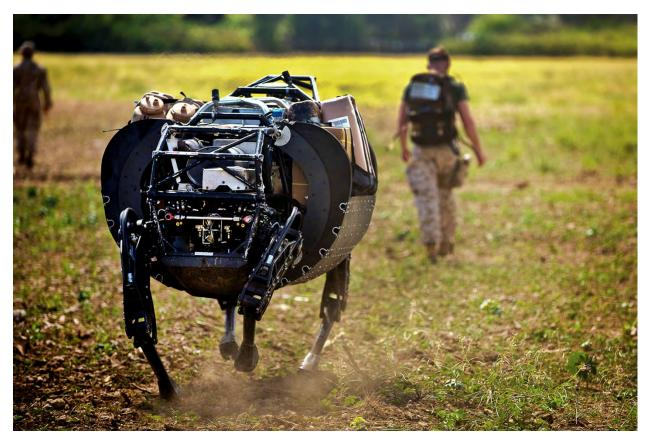
A Marine walks ahead of a legged support system at Marine Corps Training Area Bellows on Oahu, Hawaii. The legged system is designed to carry supplies, including water, food and ammunition, through rough terrain.
